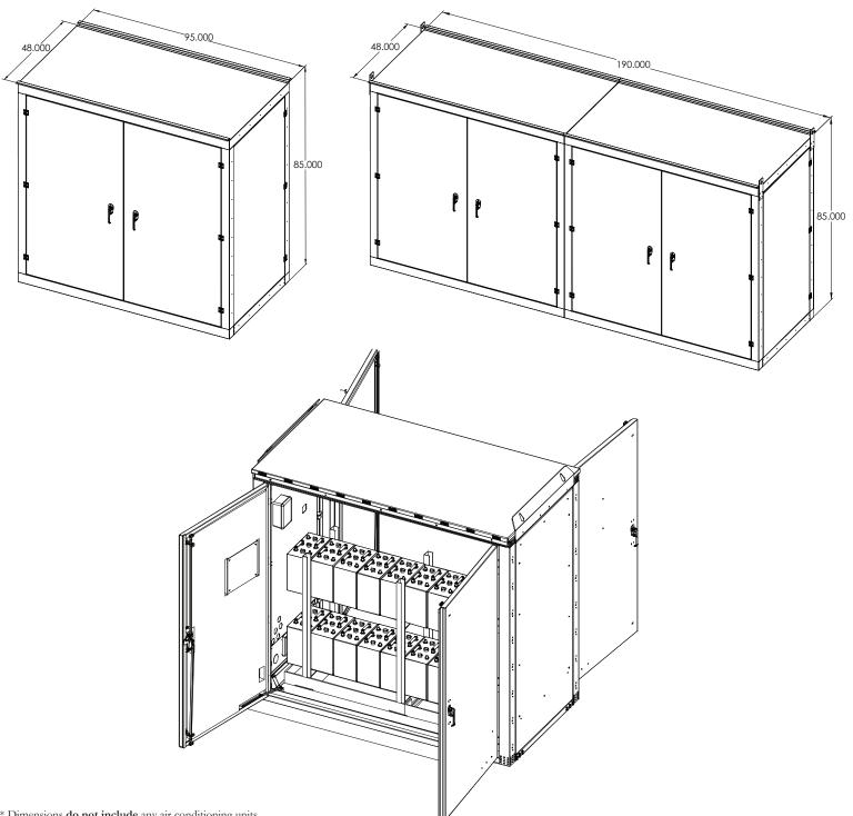
\* Dimensions <u>do not include</u> any air conditioning units. \*\* Weight <u>includes</u> a one 2,000 BTU air conditioning unit.
